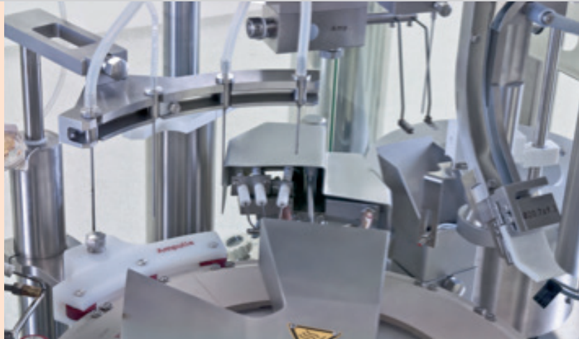
The new filling suite allows aseptic, automated fill and finish of small-volume liquid dosage forms in vials and ampoules. (Photo courtesy of Robert Bosch GmbH.)
